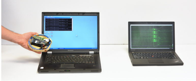
Figure 11: Untethered measurement device in online mode. The PITA (handheld) measures the target computer (left) at a specific frequency band and streams the digitized signal over WiFi, in real time, to the attacker’s computer (right). The attacker’s computer can be many meters away when using a direct WiFi connection, or (if the measurement device is configured to use a suitable WiFi access point) anywhere on the Internet.
