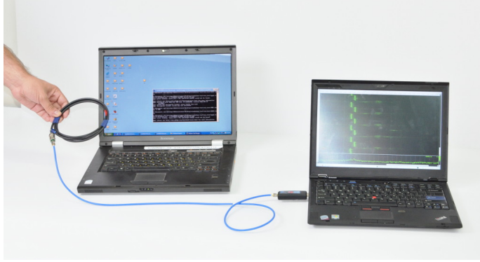
Figure 3: A shielded loop antenna (handheld) connected to the the attacker’s computer through an SDR receiver (right), attacking a Lenovo 3000 N200 target (left).
